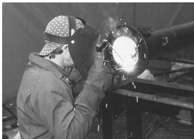
Fig. 8. Welder with appropriate personal protective equipment (NRPB 2002).
